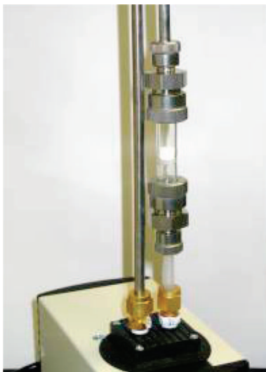
Figure 3. Packed bed reactor containing sorbent mounted on top of the recirculating pump.
