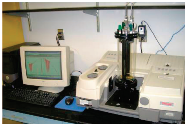
Figure 2. Long-path gas-phase IR cell, the main component of the testing apparatus.
